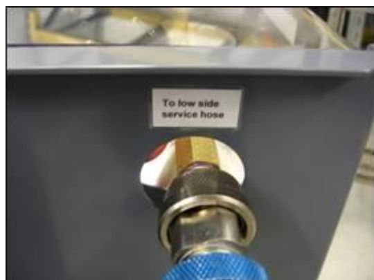
Figure 2. Example of a flushing attachment port.
